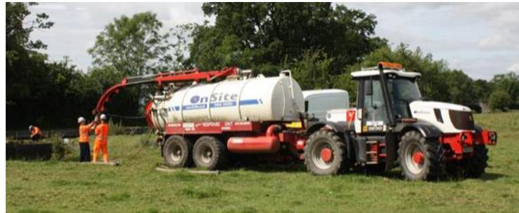
OnSite's Tractor and off road jetting unit will get to culverts where standard vans and HGV's can't. This capability often reduces the need for installing temporary roadways or line closures. Combined with our remote reel HPWJ extension there's nowhere we can't reach.
